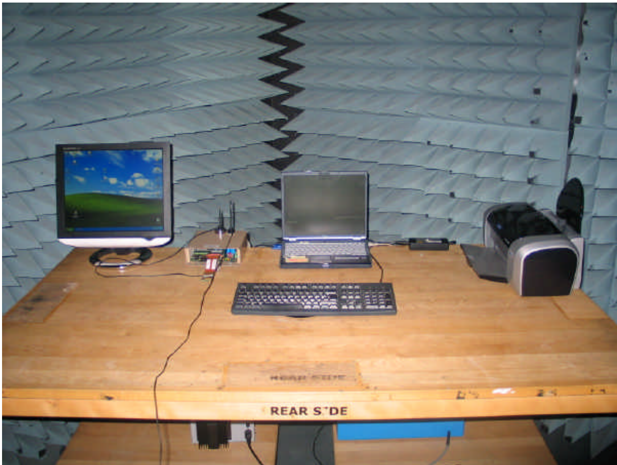
Photo 1: Test setup for radiated measurements
