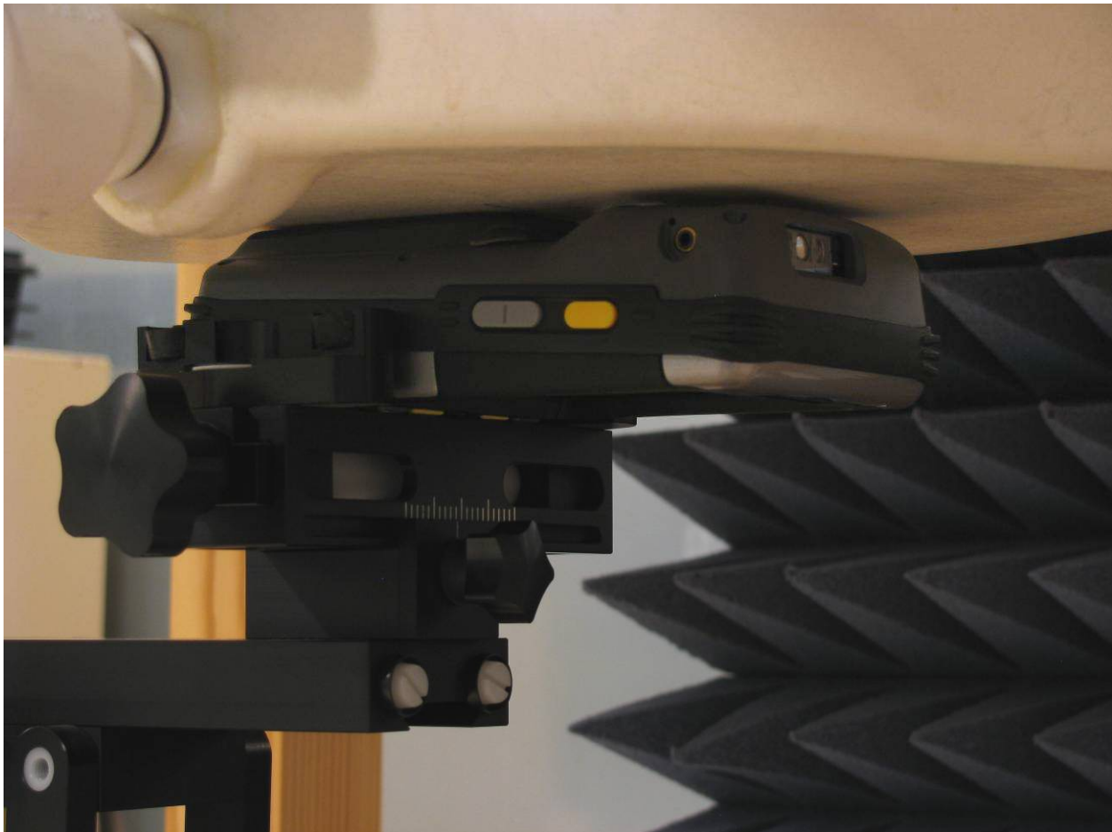
Figure 5: Device Positioning for SAR Scans
