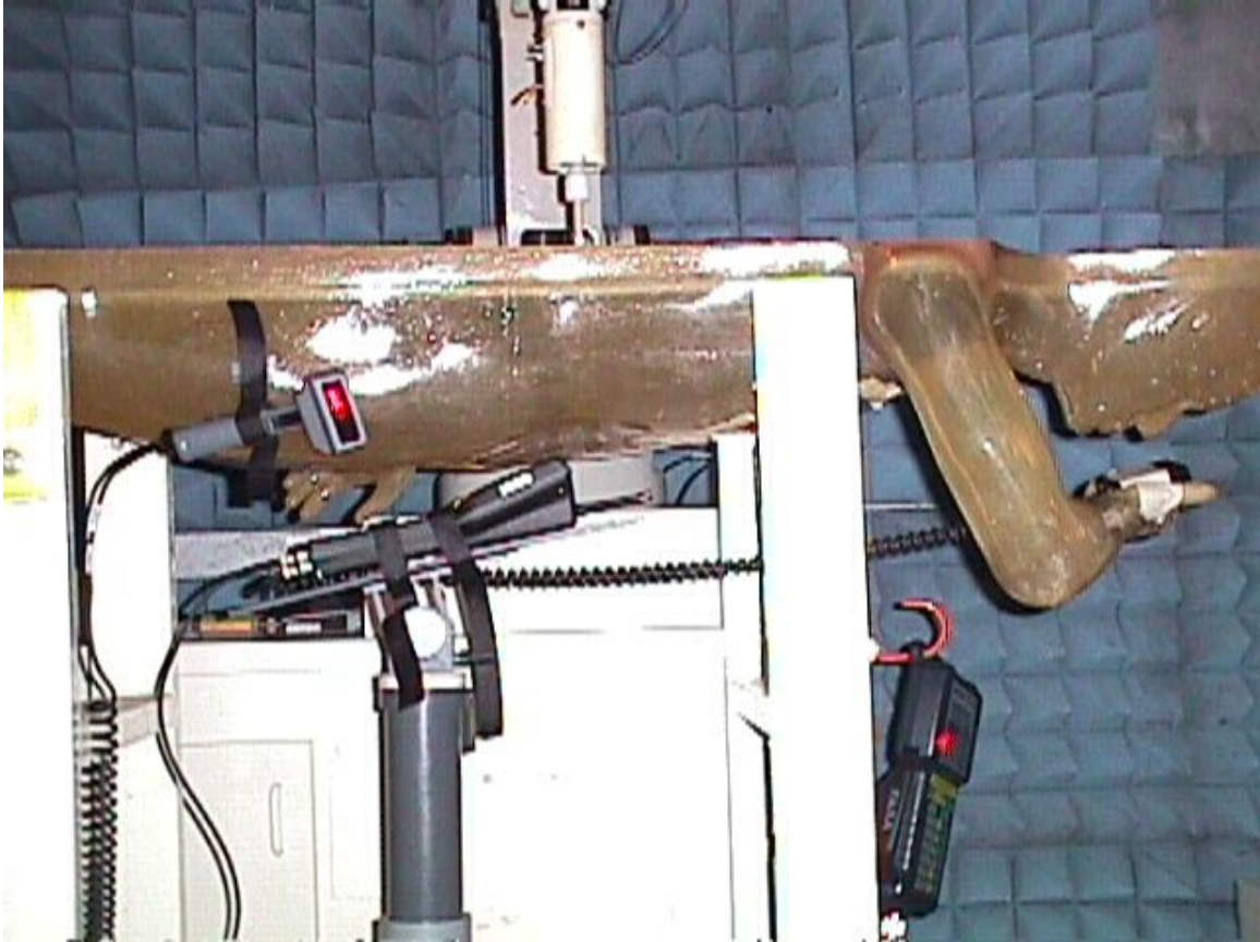
< Overview – Waist with the EUT parallel to the phantom and the display faced inward to the phantom >
