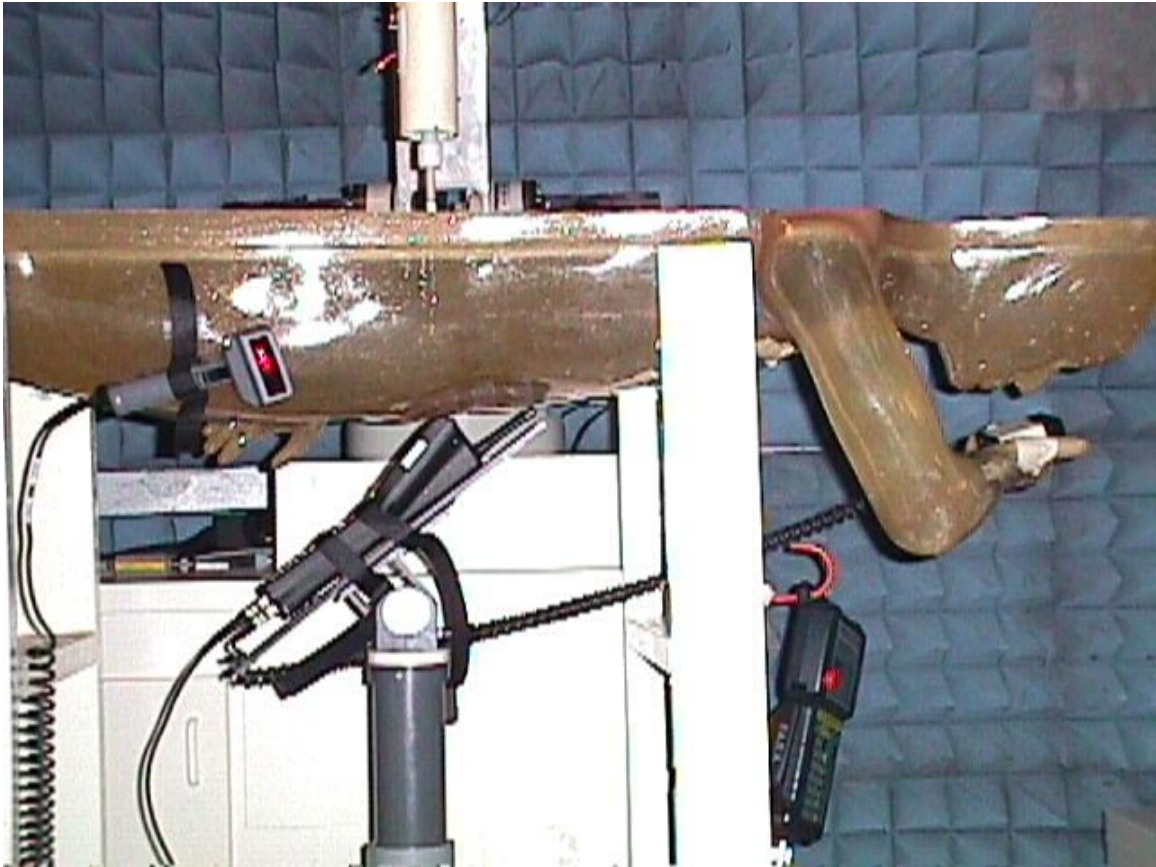
< Overview – Waist with the tip of the antenna in contact with the phantom and the display faced inward to the phantom >
