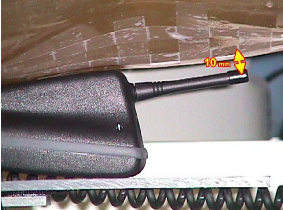
< Close-up view – Waist with the EUT parallel to the phantom and the display faced outward from the phantom >
