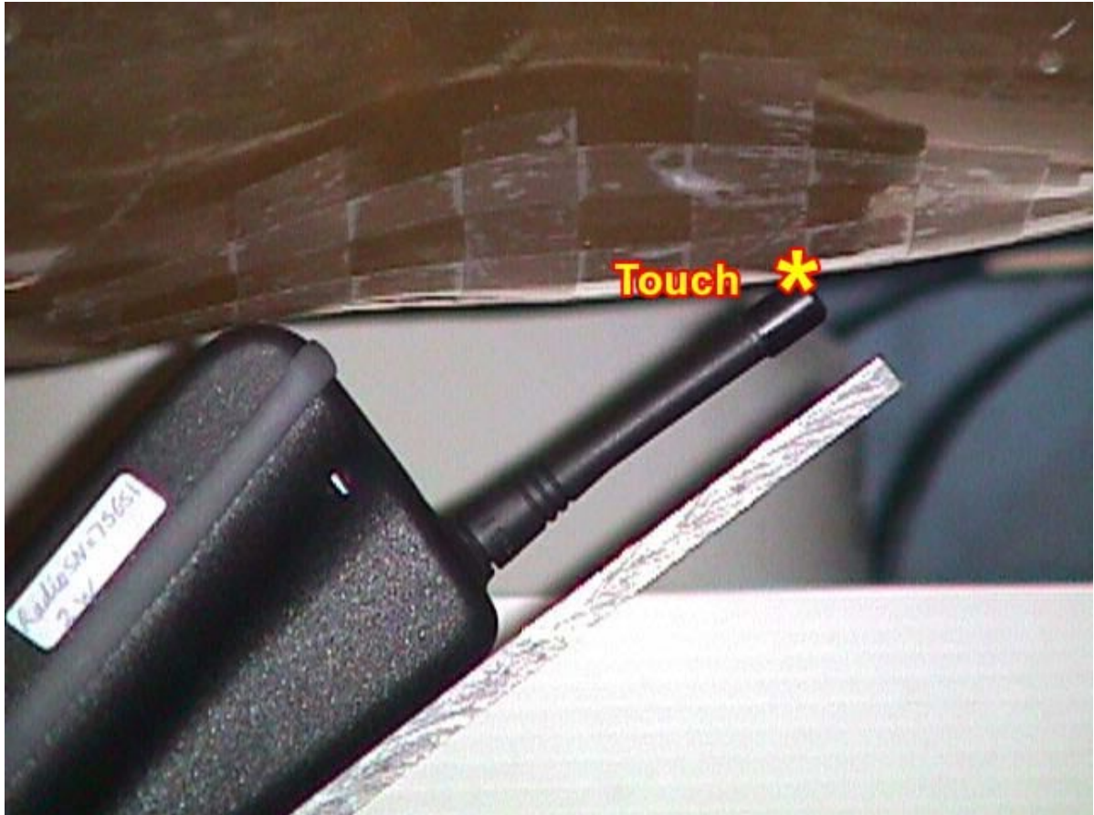
< Close-up view – Waist with the tip of the antenna in contact with the phantom and the display faced inward to the phantom >
