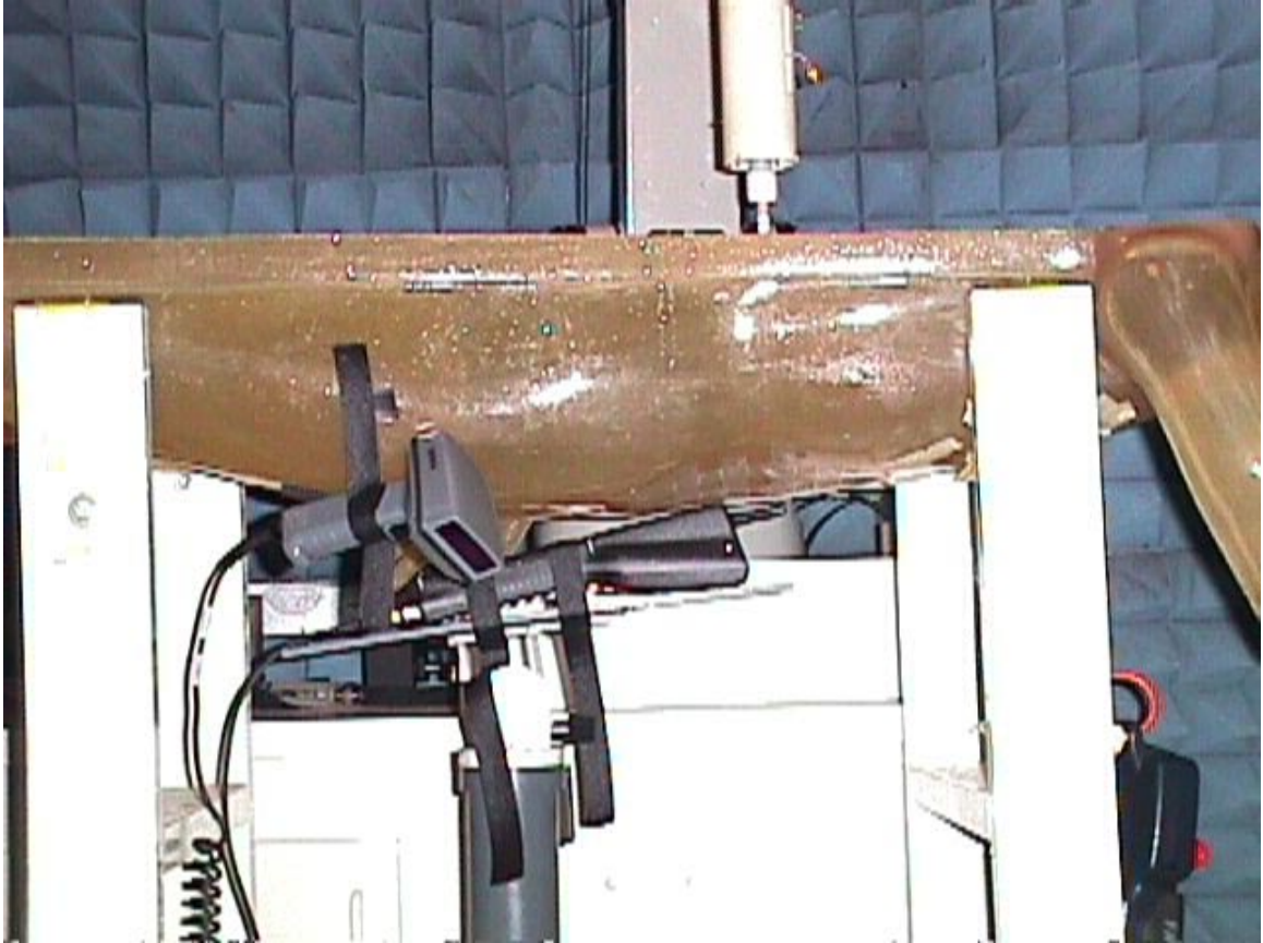
< Overview – Waist with the EUT parallel to the phantom and the display faced outward from the phantom >
