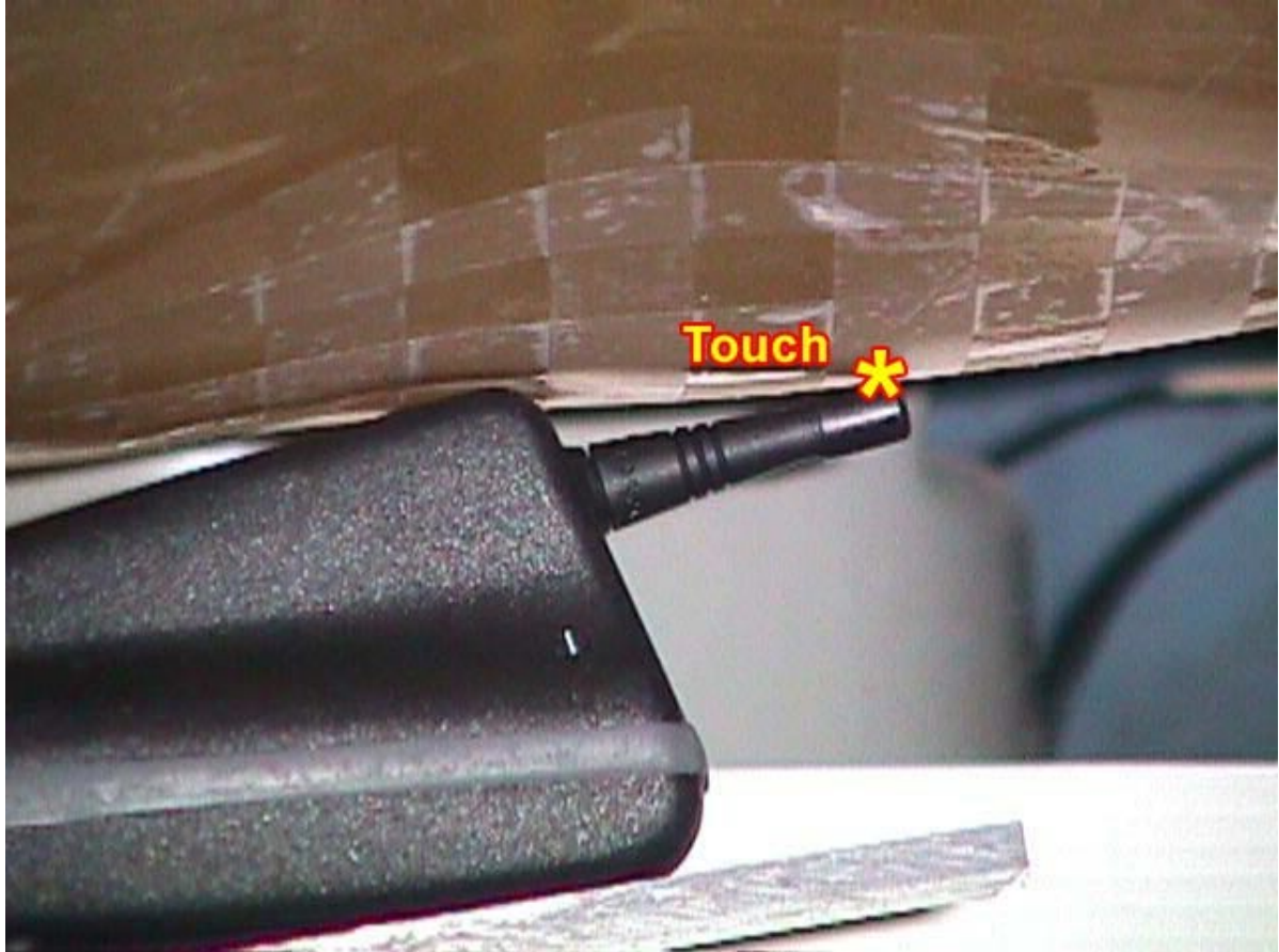
< Close-up view – Waist with the tip of the antenna in contact with the phantom and the display faced outward from the phantom >
