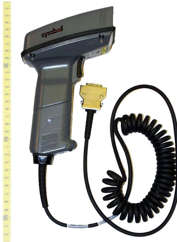
< Handheld laser scanner, M/N:LS-3200-I300A >
