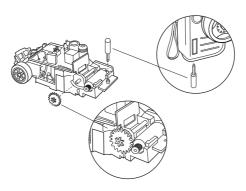
**Caution:** Do not over tighten the SET SCREW until the MOTOR CLIP WITH SET SCREW becomes slanted. It should be horizontal.
