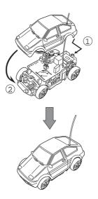
9) Thread the ANTENNA through the hold in the BODY TOP. Snap the BODY TOP to the back of the CHASSIS, and then secure the front by gently pushing the BODY TOP onto the CHASSIS as shown.
