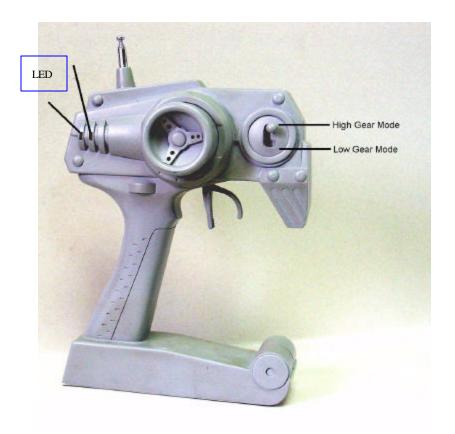
Gear Switch-Slide to control joystick up ward for High Gear Mode and down ward for Low Gear Mode
