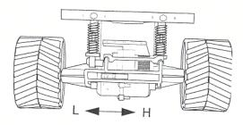
**Note**: If you cannot move **L/H** easily, slightly turn the truck's back wheels by hand. Then try again.
