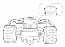
If the Agitator does not go in a straight line when you release the right control lever, use a flat-blade screwdriver to
