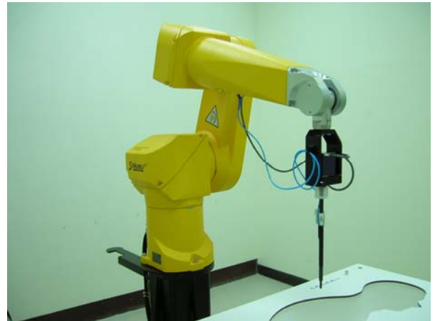
Fig. 5.2 Probe setup on robot
