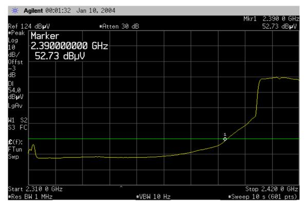
Detector mode: Peak Polarity: Horizontal
