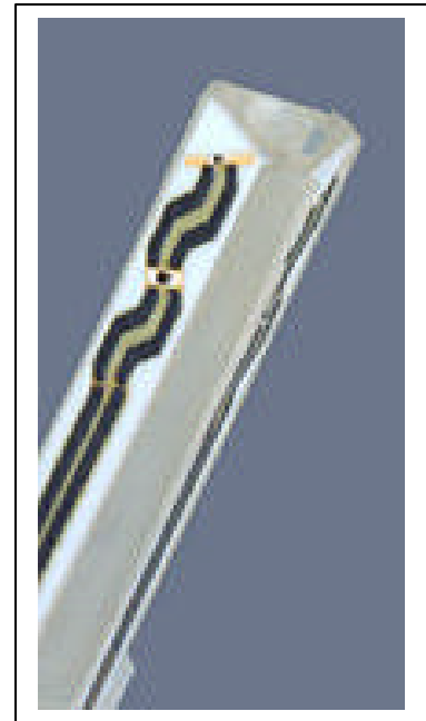
Inside view of ET3DV6 E-field Probe
