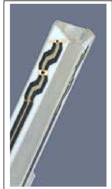
Inside view of ET3DV6 E-field Probe
