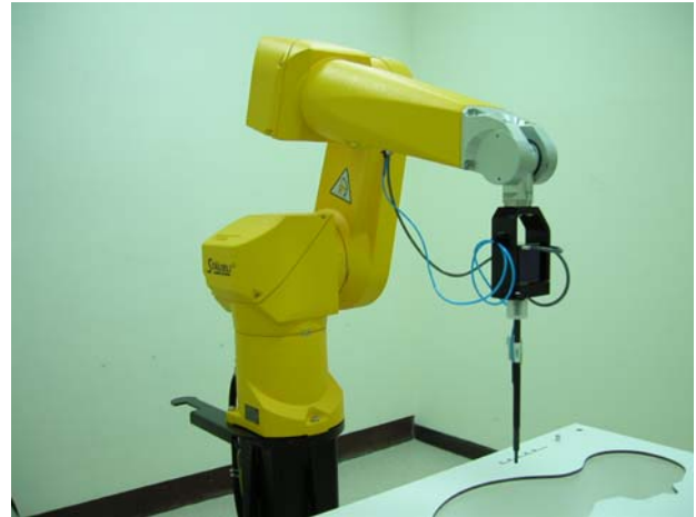
Fig. 5.2 Probe setup on robot
