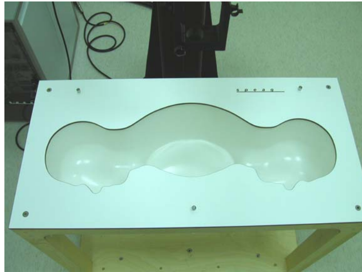
Fig. 5.3 Top view of twin phantom
