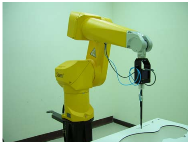
Fig. 5.2 Probe setup on robot
