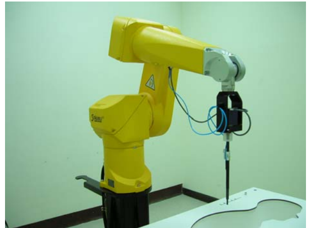
Fig. 5.2 Probe setup on robot
