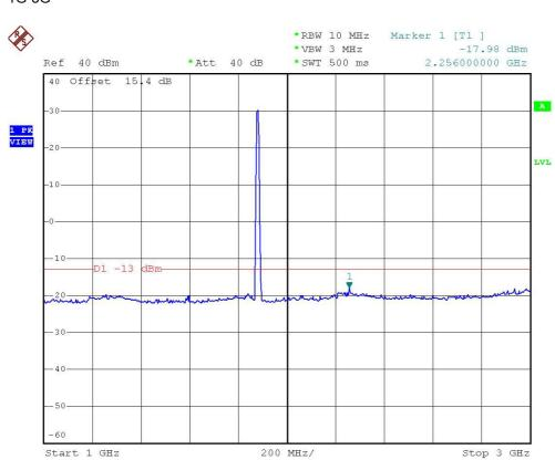
Name of Test: Conducted Spurious Emission GSM 1900 CH661 1G-3G
