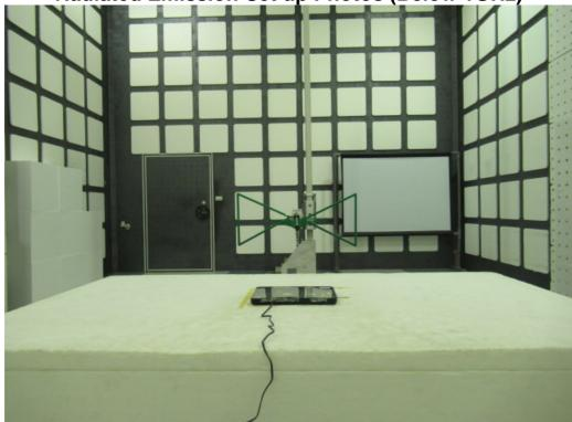
Radiated Emission Set up Photos (Above 1GHz)
