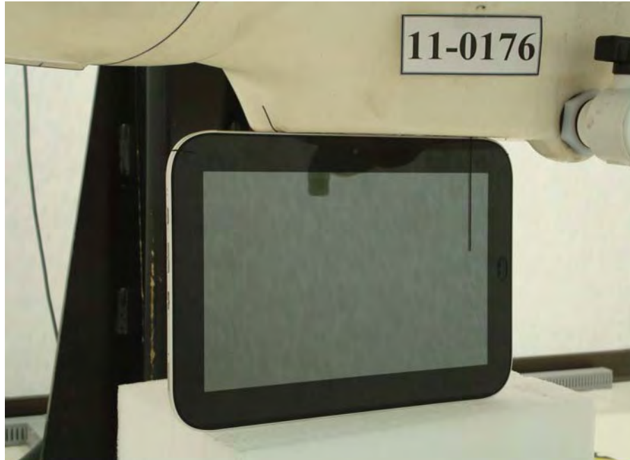
Figure 1. Body SAR Test Setup (Top Close Body)
