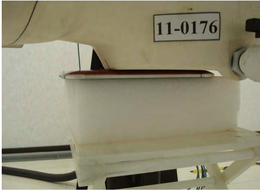
Figure 2. Body SAR Test Setup (Back Close Body)
