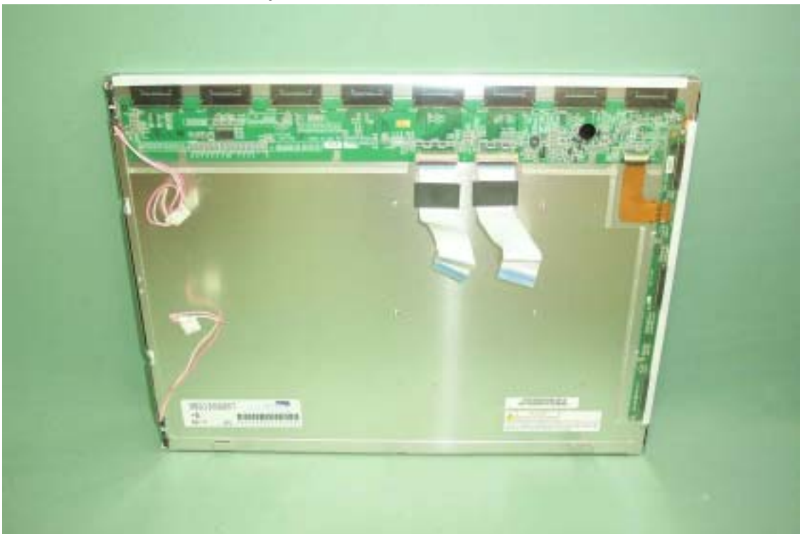
Back View of LCD Panel (HannStar/ HSD150SX87)
