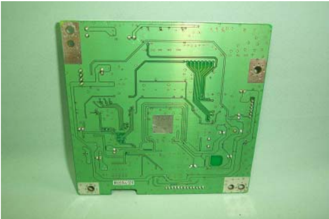
Back View of Main Board (Compal/ VL-575)
