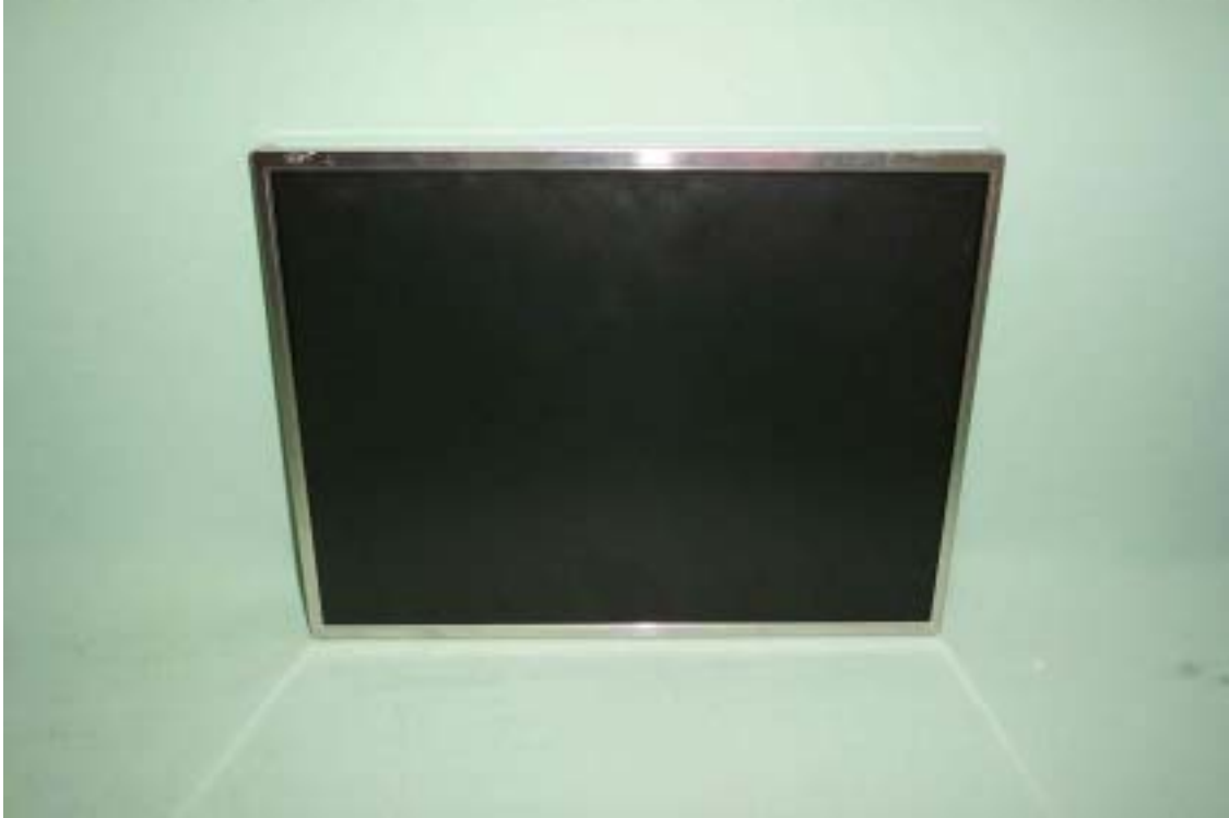
Back View of LCD Panel (HannStar/ HSD150SX87)
