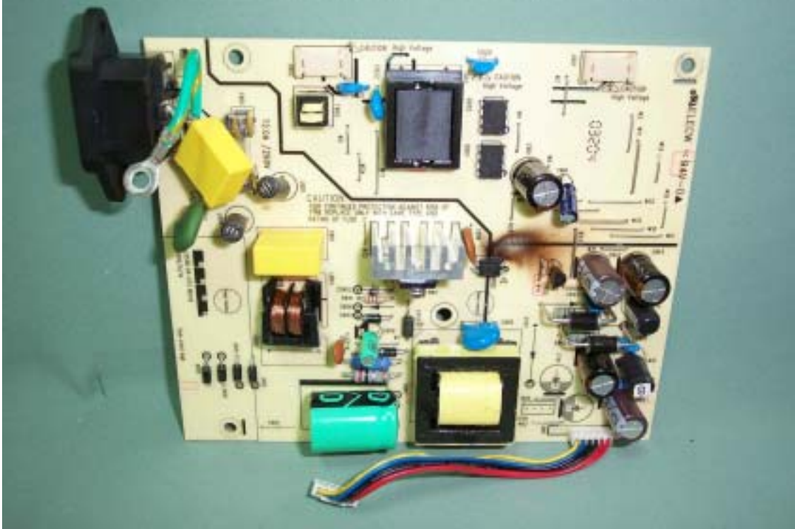
Back View of Power Board (Compal/ VP-575)
