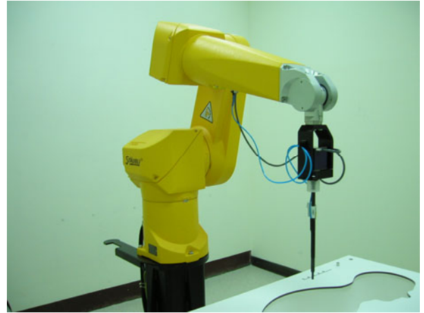
Fig. 5.2 Probe setup on robot
