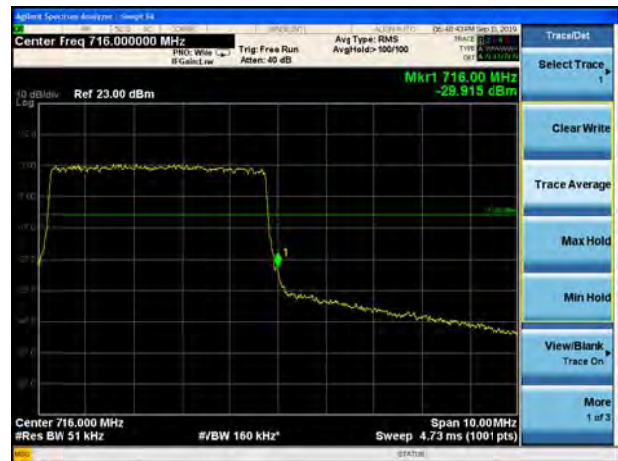
LTE Band 12 16QAM 10MHz CH-High, 1 RB
