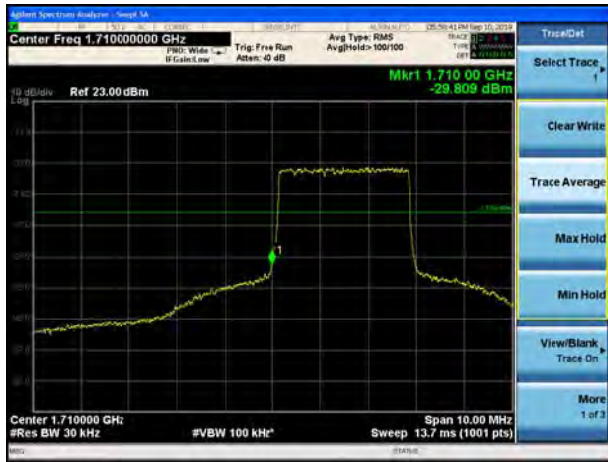
LTE Band 4 16QAM 5MHz CH-Low, 1 RB
