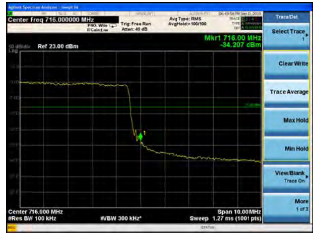
LTE Band 13 QPSK 5MHz CH-High, 1 RB
