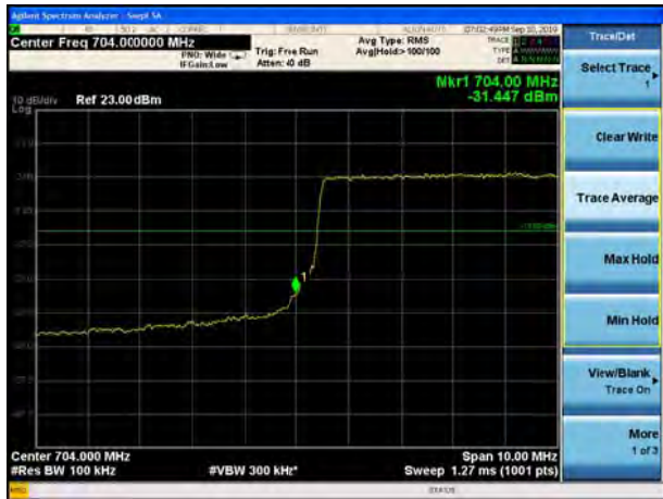
LTE Band 17 16QAM 5MHz CH-Low, 1 RB
