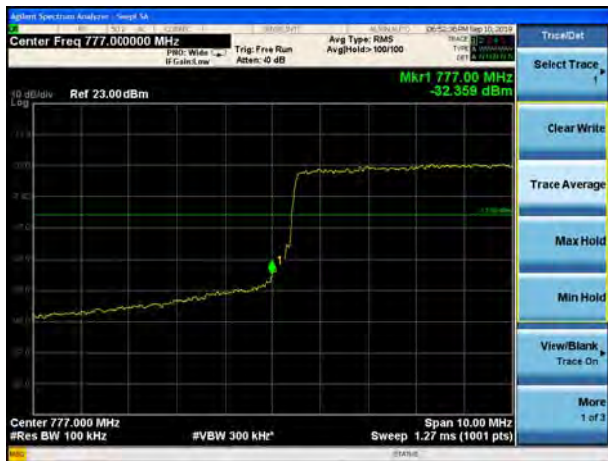
LTE Band 13 16QAM 5MHz CH-Low, 1 RB
