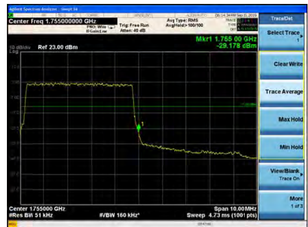
LTE Band 4 QPSK 5MHz CH-High, 100%RB
