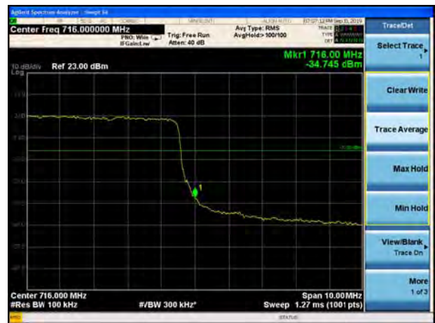
LTE Band 17 16QAM 10MHz CH-High, 100%RB
