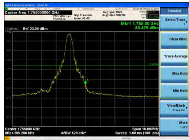
LTE Band 4 16QAM 20MHz CH-High, 100%RB
