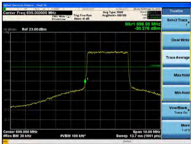
LTE Band 12 16QAM 3MHz CH-Low, 100%RB
