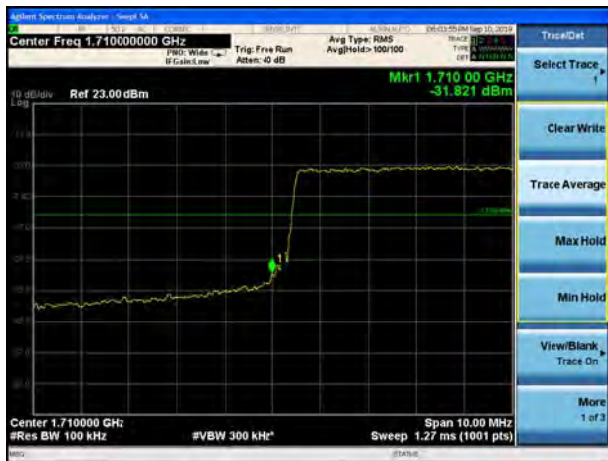
LTE Band 4 QPSK 15MHz CH-Low, 1 RB
