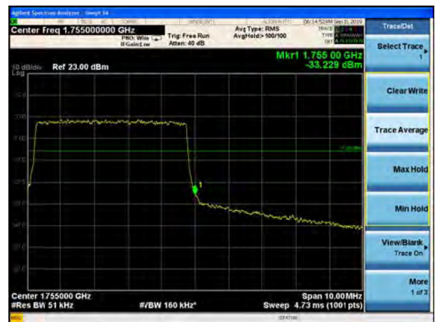
LTE Band 4 16QAM 5MHz CH-High, 100%RB
