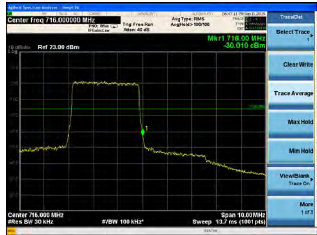
LTE Band 12 QPSK 5MHz CH-High, 1 RB
