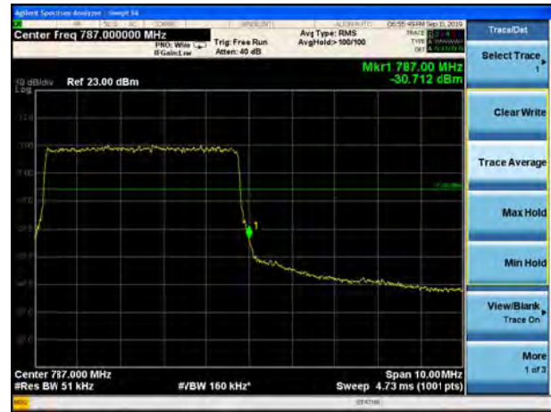
LTE Band 13 16QAM 10MHz CH-High, 1 RB
