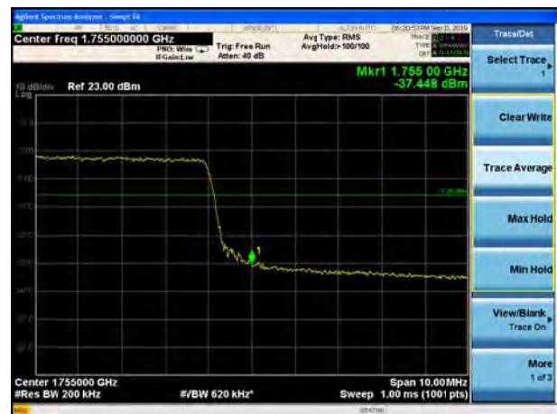
LTE Band 4 16QAM 20MHz CH-High, 100%RB
