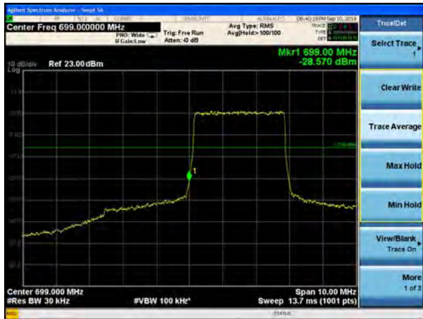
LTE Band 12 QPSK 5MHz CH-Low, 1 RB
