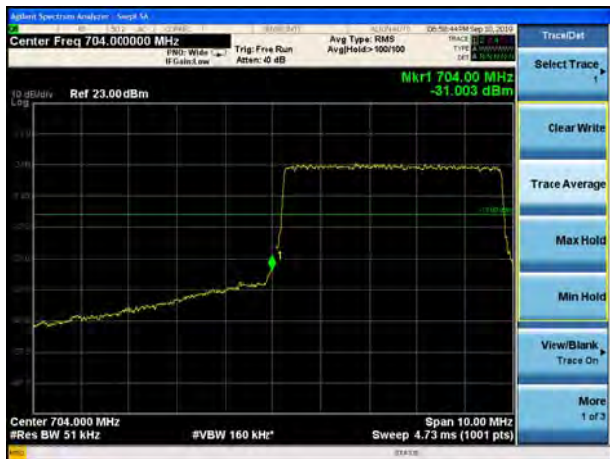
LTE Band 17 16QAM 5MHz CH-Low, 100%RB
