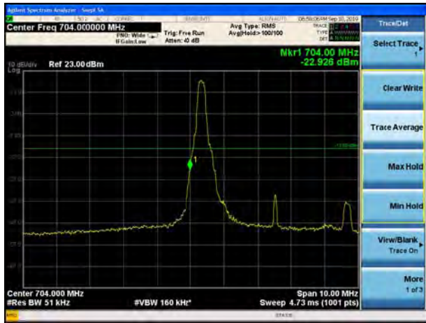
LTE Band 17 QPSK 5MHz CH-Low, 100%RB
