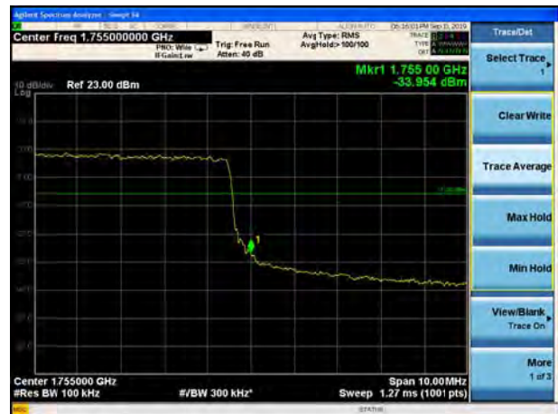
LTE Band 4 16QAM 15MHz CH-High, 1 RB
