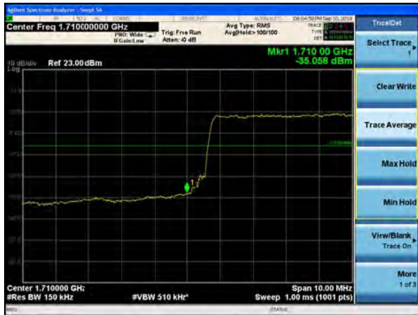
LTE Band 4 QPSK 20MHz CH-Low, 1 RB
