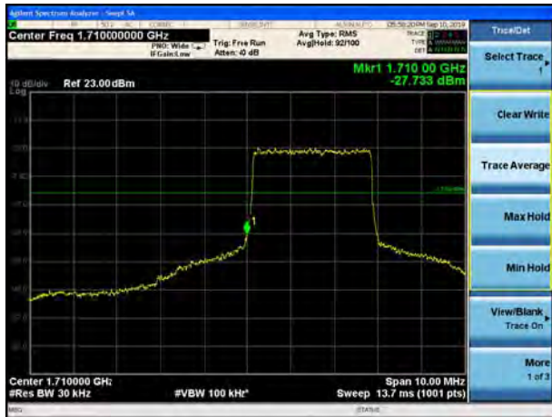
LTE Band 4 QPSK 5MHz CH-Low, 1 RB
