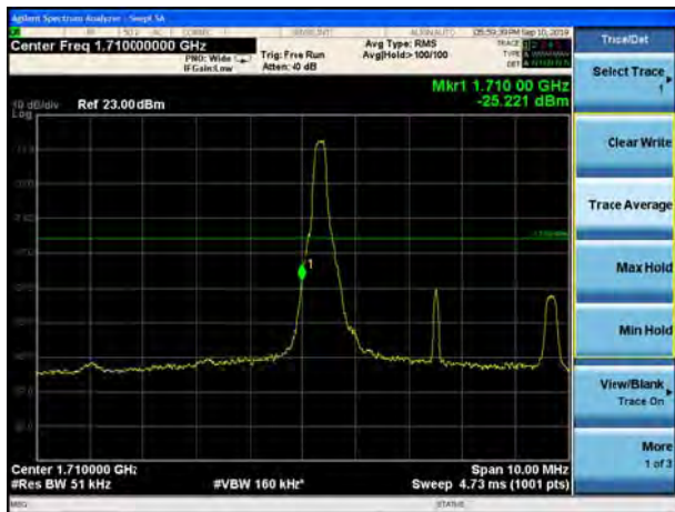
LTE Band 4 16QAM 5MHz CH-Low, 100%RB
