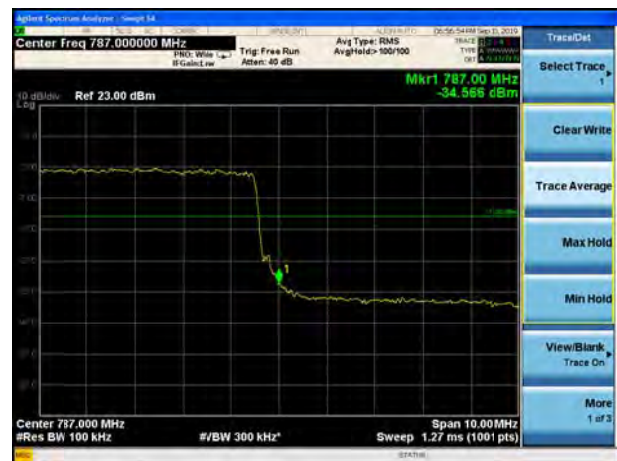
LTE Band 13 16QAM 10MHz CH-High, 100%RB
