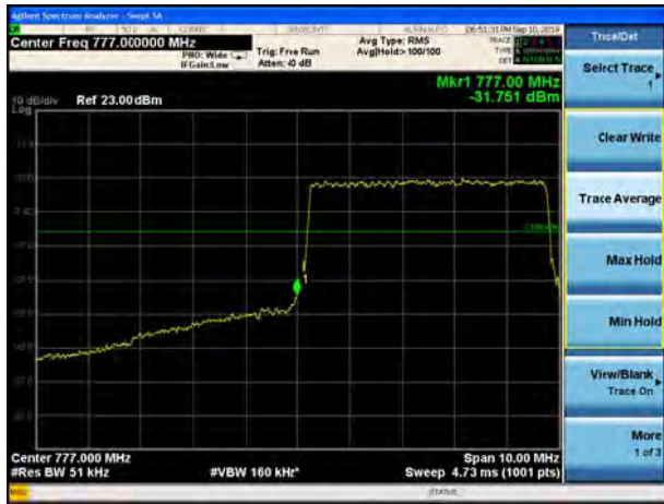
LTE Band 13 16QAM 10MHz CH-Low, 1 RB
