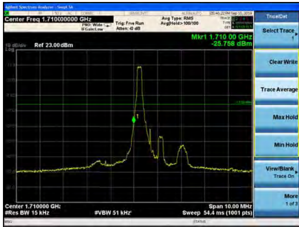
LTE Band 4 QPSK 1.4MHz CH-Low, 100%RB
