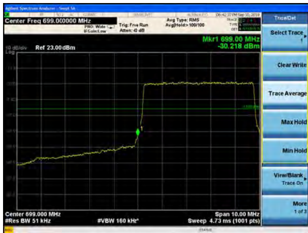
LTE Band 12 QPSK 5MHz CH-Low, 100%RB
