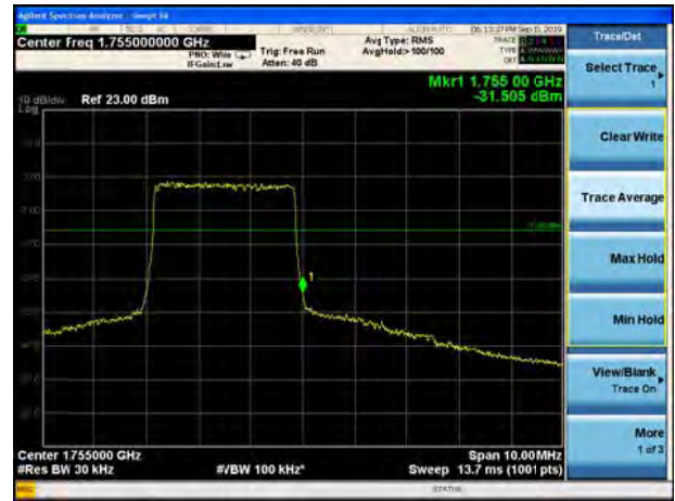
LTE Band 4 16QAM 5MHz CH-High, 1 RB
