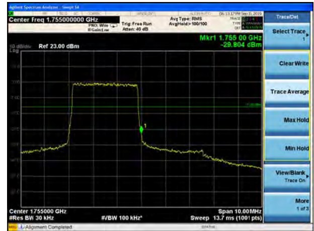
LTE Band 4 QPSK 5MHz CH-High, 1 RB
