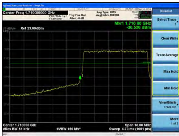
LTE Band 4 16QAM 5MHz CH-Low, 100%RB
