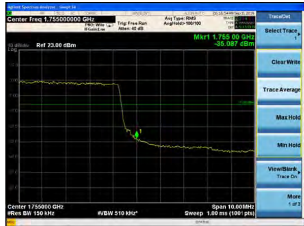
LTE Band 4 QPSK 20MHz CH-High, 1 RB
