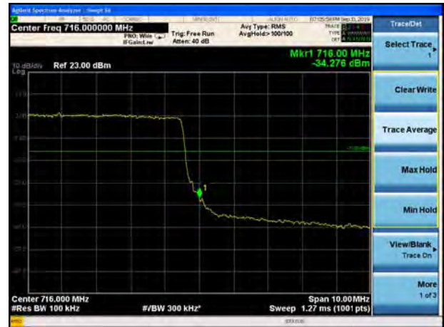
LTE Band 17 16QAM 5MHz CH-High, 1 RB
