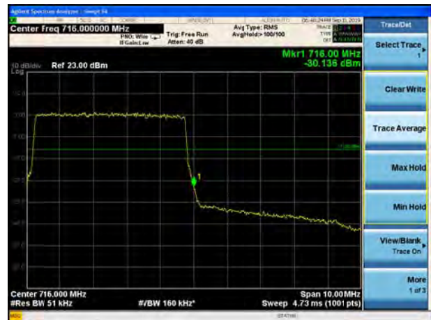
LTE Band 12 QPSK 5MHz CH-High, 100%RB
