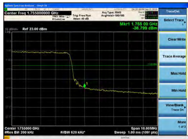
LTE Band 4 QPSK 20MHz CH-High, 100%RB
