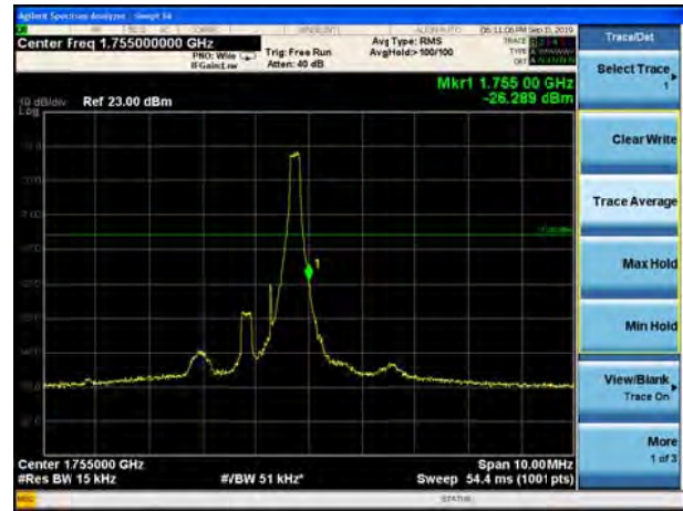
LTE Band 4 16QAM 1.4MHz CH-High, 100%RB
