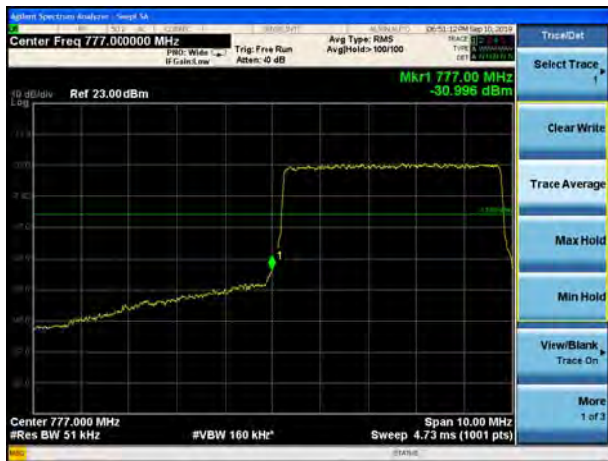
LTE Band 13 QPSK 5MHz CH-Low, 100%RB
