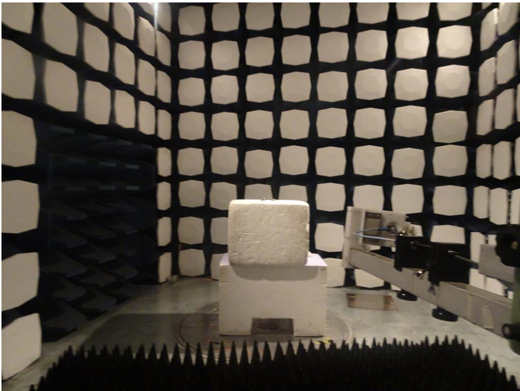
Picture 1: Radiated Spurious Emissions Test setup
