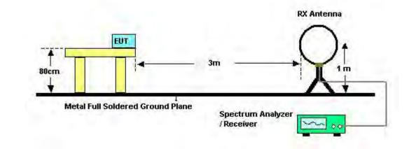
For Radiated Emissions: 30MHz~1GHz
