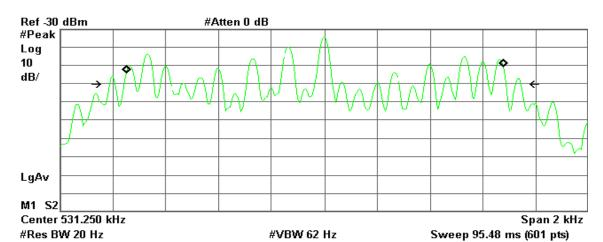
Occupied Bandwidth 1.4240 kHz Occ BW % Pwr 99.00 % -26.00 dB x dB
