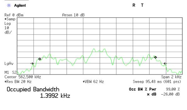
Transmit Freq Error -25.064 Hz x dB Bandwidth 1.509 kHz\*
