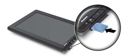
When a flash media card is inserted into the 3-in-1 media card reader, a pop-up message is displayed asking if you want to display the contents on the card. To display the contents, touch **Start Utility**. Otherwise, touch **Don't start**.
