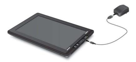
Figure 7. Connecting the ac charger with the tablet
