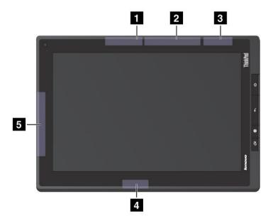
Figure 17. Location of the UltraConnect wireless antennas
