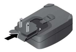
Figure 6. Installing the ac charger
