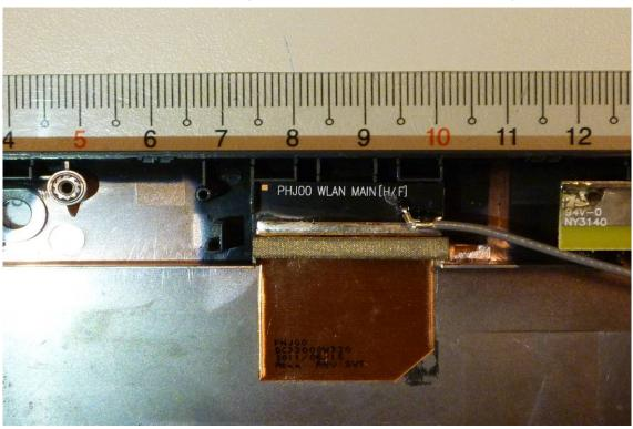
Antenna location (WLAN and BT AUX Antenna, model: Acon)
