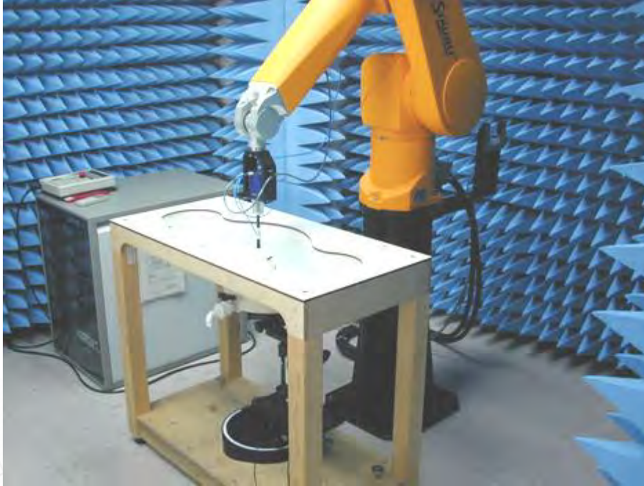
Fig.1 Photograph of the SAR measurement System
