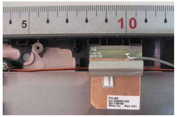
WLAN and BT AUX Antenna
