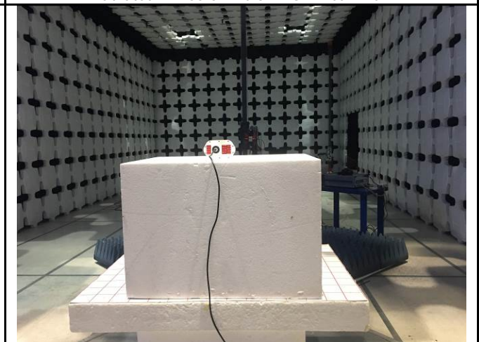
Radiated Emission Above 1G - Rear View
