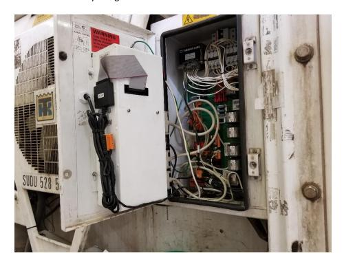
11. Close the asset door. The device should be oriented as pictured below:
