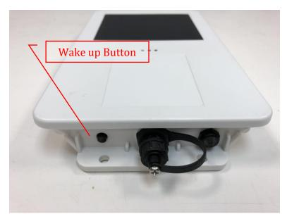
**Note:** The factory default settings are configured to have the device to sleep within 2 minutes of wake. Consider pulling the IN1 wire high to keep the device awake for configuration purposes or disable sleep by issuing the proper 3017 command.
