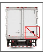
• Avoid mounting the XT4975A to locations that are high risk to predictable physical harm. (I.e. do not mount the unit on the top of an asset if snow scrapers are utilized in periodic maintenance of the asset without some sort of protective bracket)
