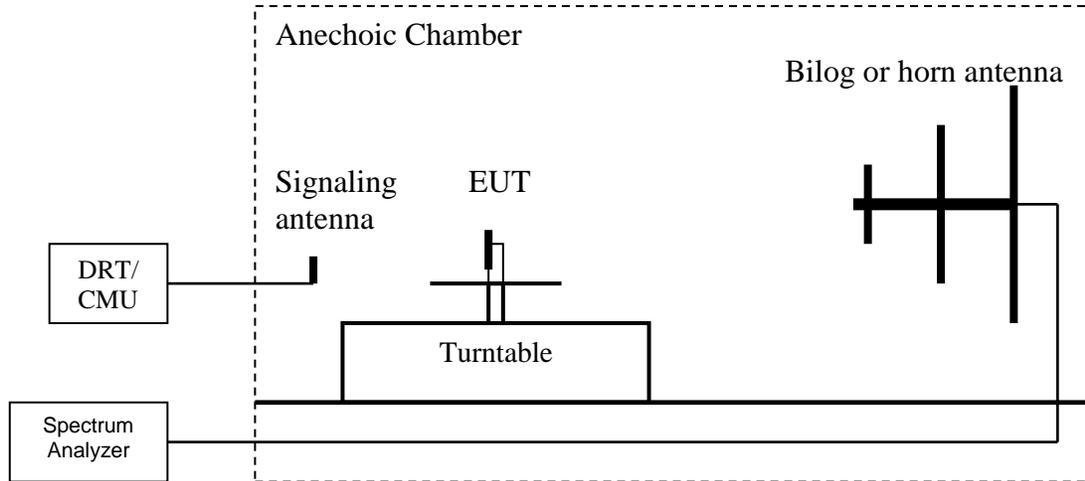
Connect the equipment as shown in the above diagram with the EUT's antenna in center of the turn table.
