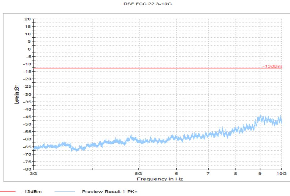
**Test results – 3GHz – 10GHz -High Channel (GSM850)**
