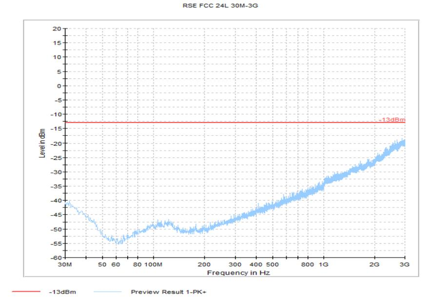
**Test results 30MHz-3GHz – Mid Channel (GSM-1900)**
