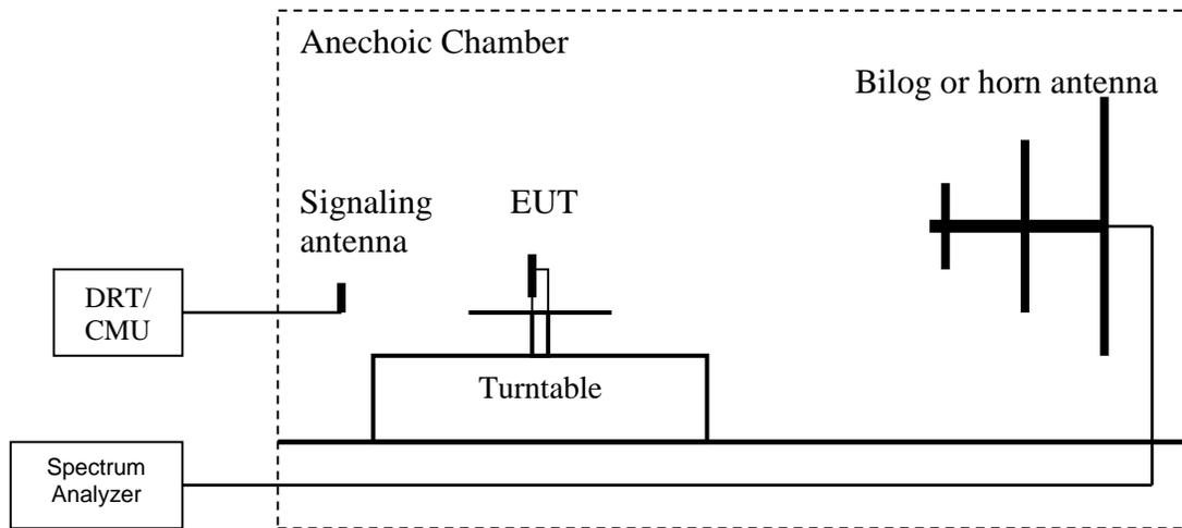
Connect the equipment as shown in the above diagram with the EUT's antenna in a horizontal orientation.
