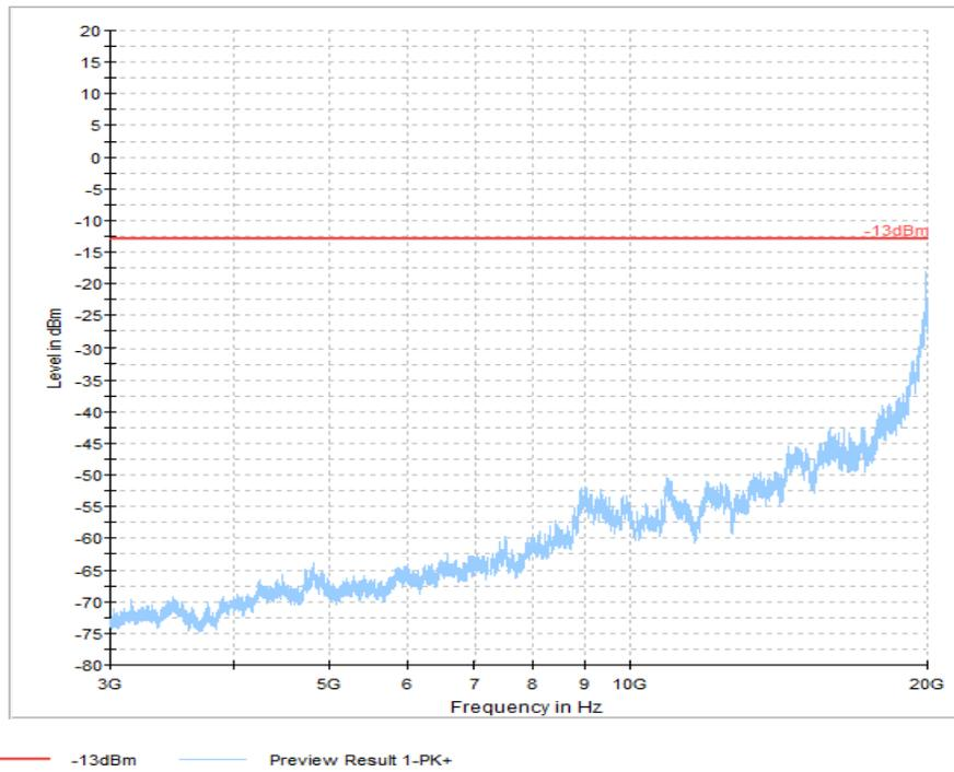
**Radiated Spurious Emissions (UMTS Band 5) Tx:**
