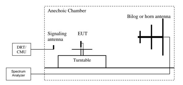
Connect the equipment as shown in the above diagram with the EUT's antenna in center of the turn table.
