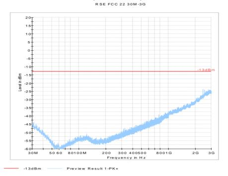
Test results 30 MHz-1GHz – Mid Channel (UMTS-Band 5)
