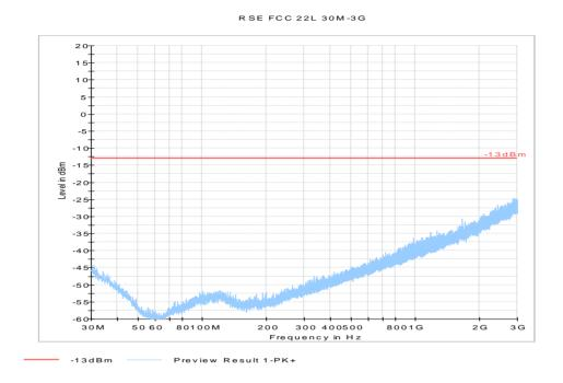
Test results - 30 MHz – 3GHz -Mid Channel (GSM850)
