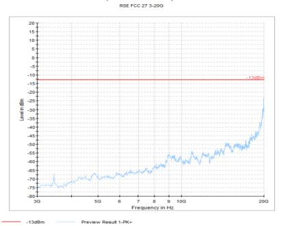
Test results 3GHz-20GHz– High Channel (UMTS-Band 4)
