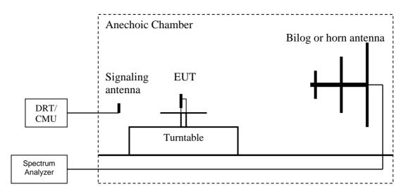
Connect the equipment as shown in the above diagram with the EUT's antenna in a horizontal orientation.
