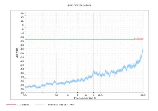
Test results 3 GHz-20 GHz – Mid Channel (GSM-1900)
