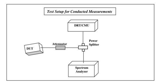
Connect the equipment as shown in the above diagram. A Digital Radio Communication Tester (DRT: R&S CMU200 here) is used to enable the EUT to transmit and to measure the output power.
