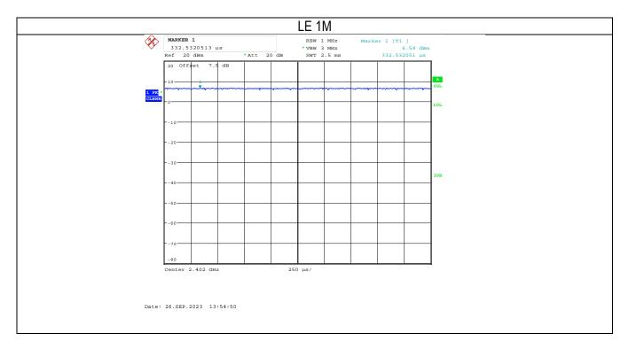
**Note**: The EUT operates at a 100% duty cycle using the Direct Test Mode firmware, exclusively for compliance testing. In contrast, regular production units are set to a maximum 20% duty cycle for BTLE 1Mbps. For Radiated Spurious Emissions testing, a correction factor for the duty cycle will be used to convert the MaxPeak measurement outcome to the Average result.
