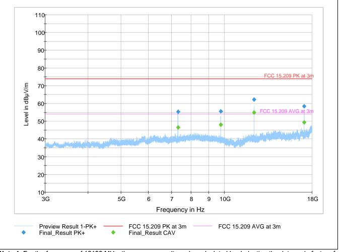
**Note 1**: For the frequency of 12199 MHz, the average result can be calculated by deducting the duty cycle factor of 13.98dBuV/m from the peak result of 62.110dBuV/m, yielding 48.13dBuV/m. This result remains below the average limit of 53.98dBuV/m.
