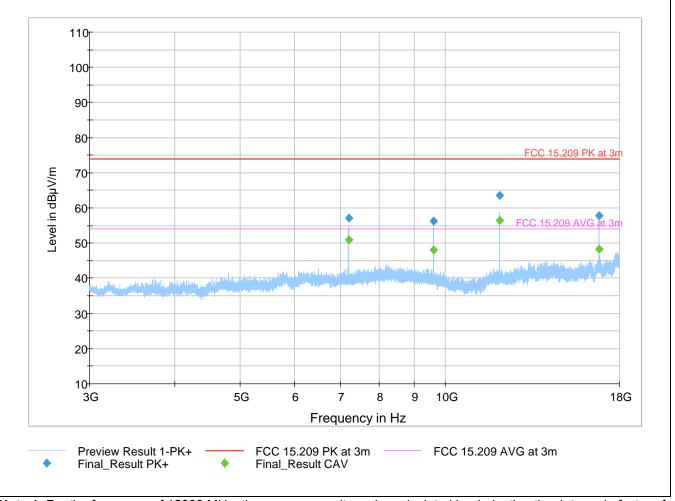
**Note 1**: For the frequency of 12009 MHz, the average result can be calculated by deducting the duty cycle factor of 13.98dBuV/m from the peak result of 63.506dBuV/m, yielding 49.526dBuV/m. This result remains below the average limit of 53.98dBuV/m.
