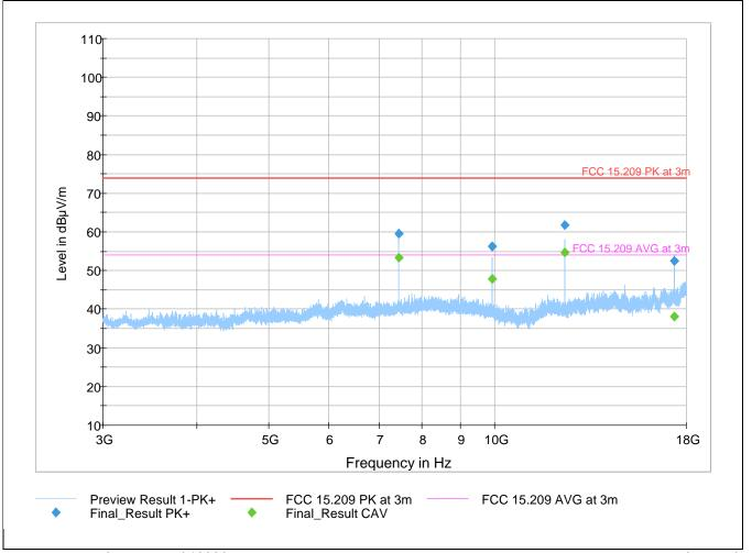
**Note 1**: For the frequency of 12399 MHz, the average result can be calculated by deducting the duty cycle factor of 13.98dBuV/m from the peak result of 61.873dBuV/m, yielding 47.893dBuV/m. This result remains below the average limit of 53.98dBuV/m.
