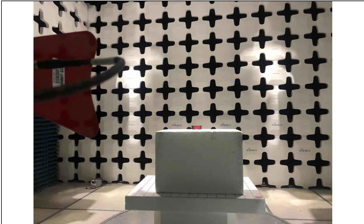
Radiated Emission Test above 1GHz Front View
