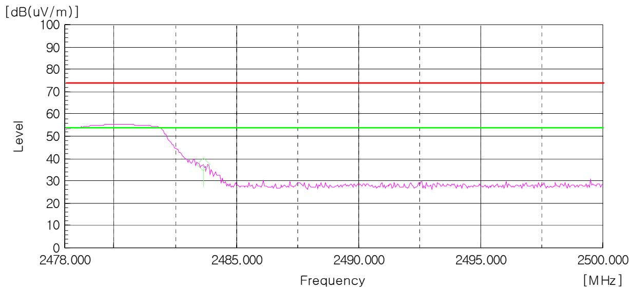
AV Detector: RBW: 1MHz, VBW: 10 Hz (2 483.5 MHz - 2 500.0 MHz), Worst case (High, Horizontal)
