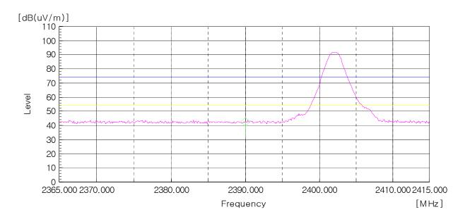
AV Detector: RBW: 1 MHz, VBW: 10 Hz (2 365 MHz - 2 415 MHz), Worst case (Low, Horizontal)
