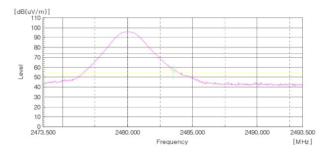
AV Detector: RBW: 1MHz, VBW: 10 Hz (2 473.5 MHz - 2 493.5 MHz), Worst case (High, Horizontal)
