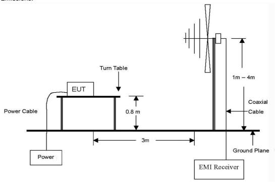
The diagram below shows the test setup that is utilized to make the measurements for emission .The spurious emissions were investigated form 1 % to the 10th harmonic of the highest fundamental frequency or 40 %, whichever is lower.
