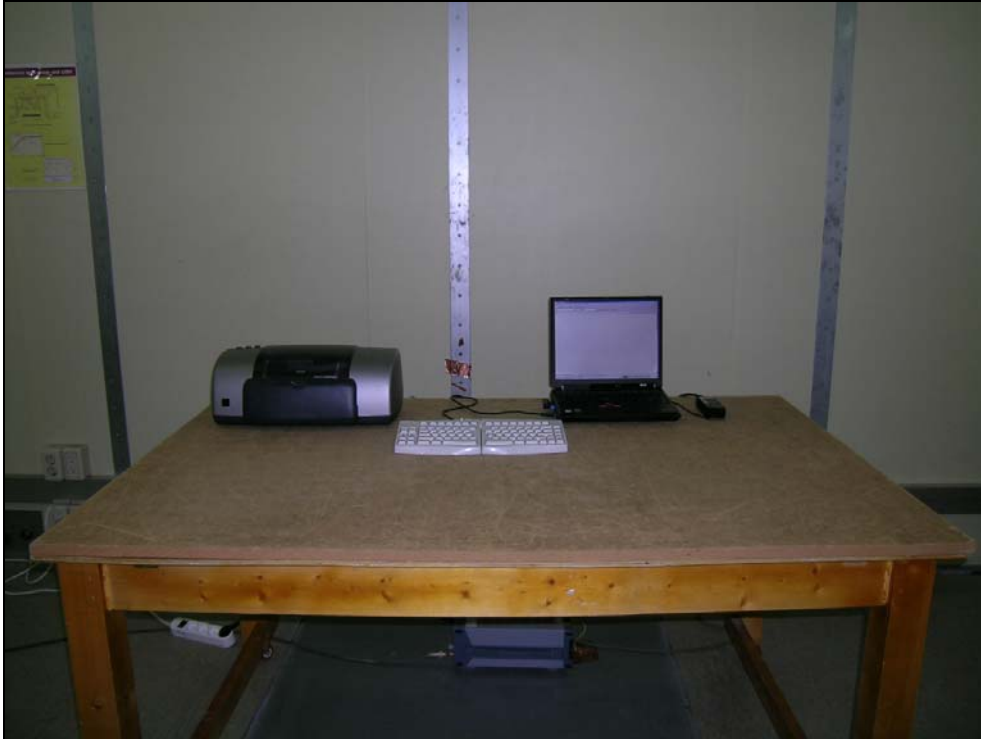
Photograph 1: Setup for Conducted Emissions
