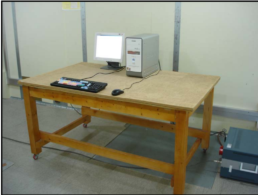
Photograph 1: Setup for Conducted Emissions
