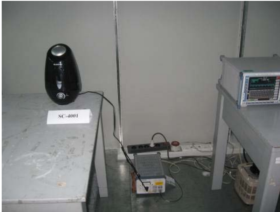
Photograph 1: Set-up for Conducted Emission
