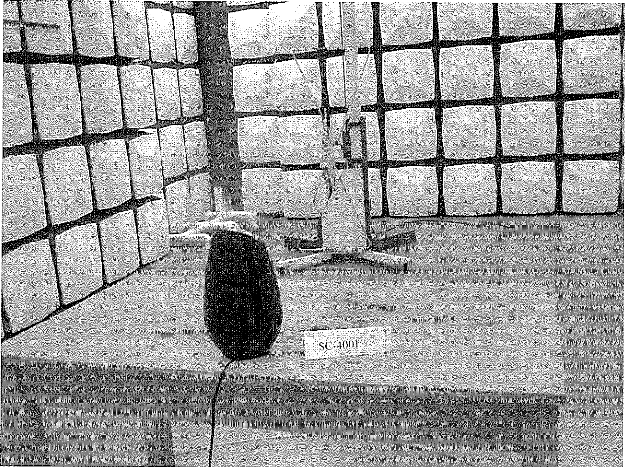
Photograph 2: Set-up for Radiated Emission
