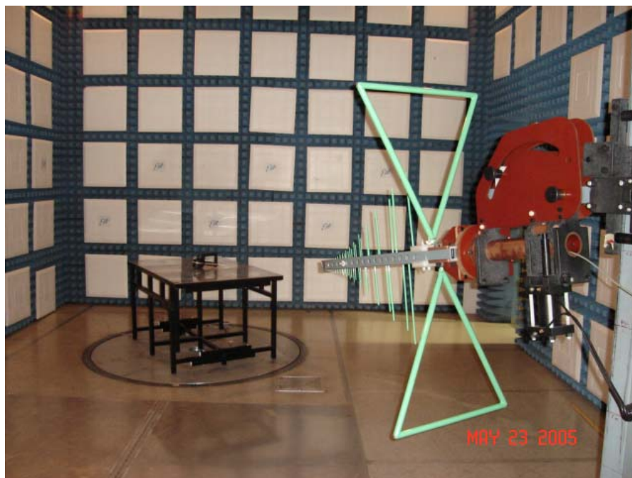
Test Setup for Measurement of Radiated Emissions
