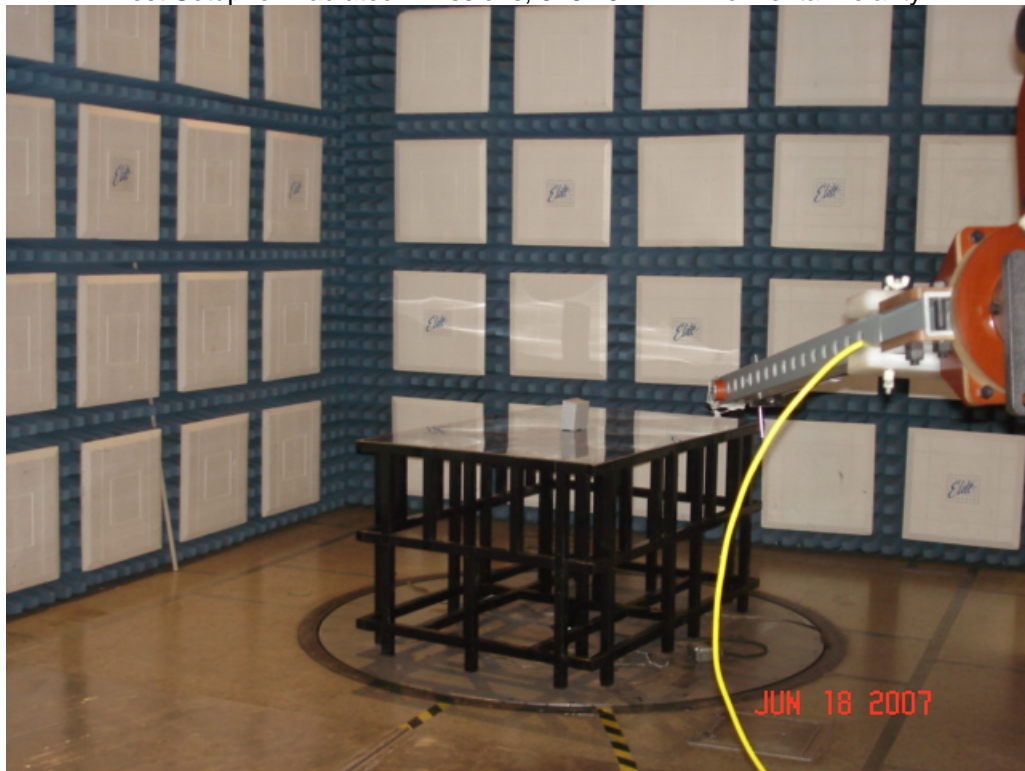
Test Setup for Radiated Emissions, 916.45MHz – Vertical Polarity
