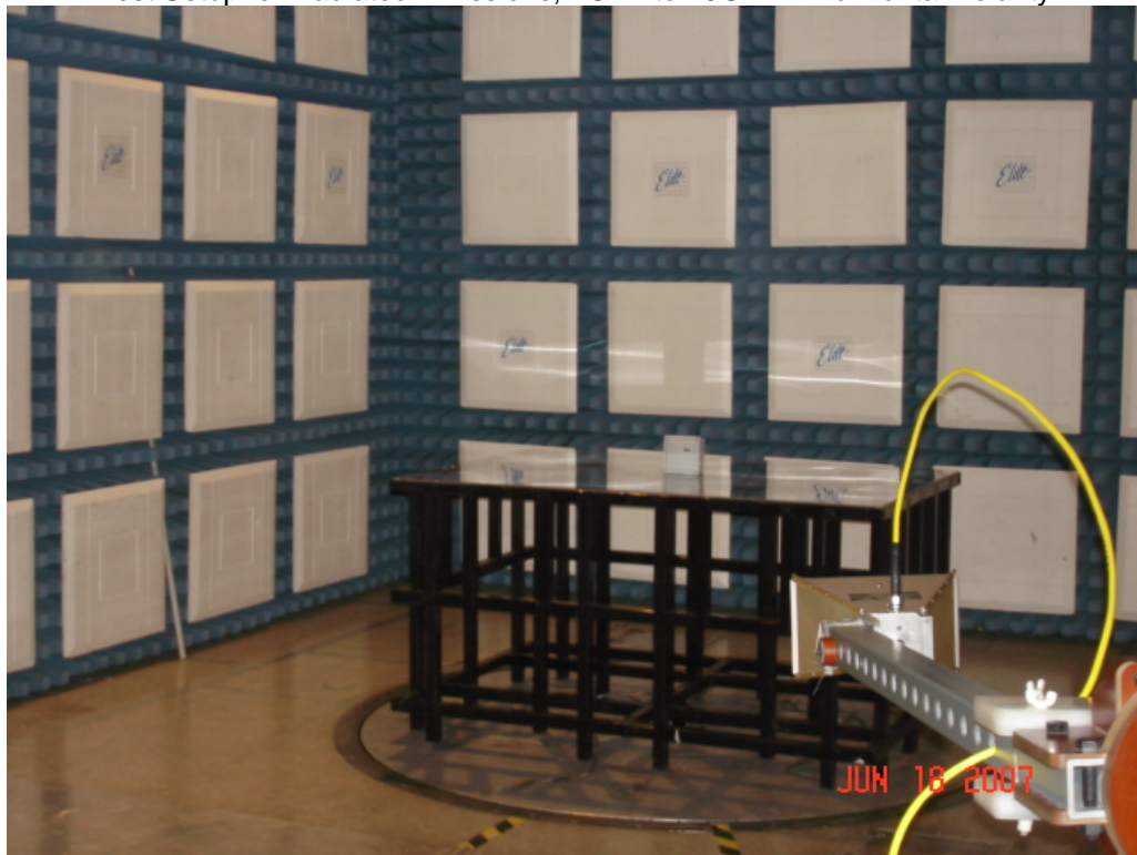
Test Setup for Radiated Emissions, 1GHz to 10GHz – Vertical Polarity
