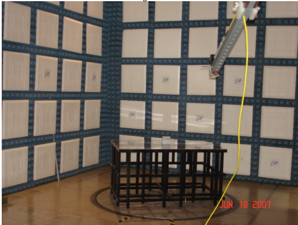
Test Setup for Radiated Emissions, 916.45MHz – Horizontal Polarity
