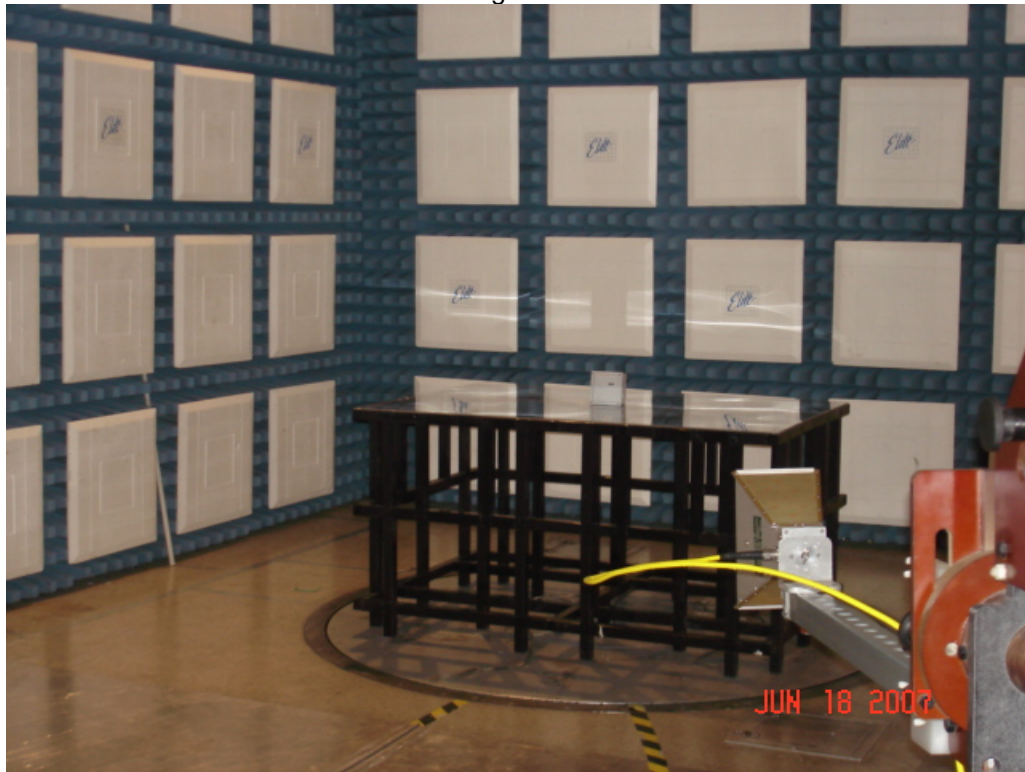
Test Setup for Radiated Emissions, 1GHz to 10GHz – Horizontal Polarity
