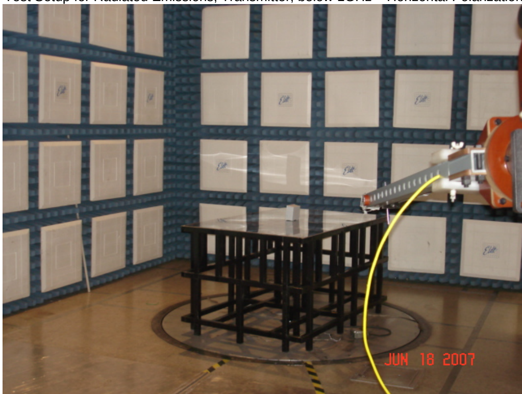
Test Setup for Radiated Emissions, Transmitter below 1GHz – Vertical Polarization
