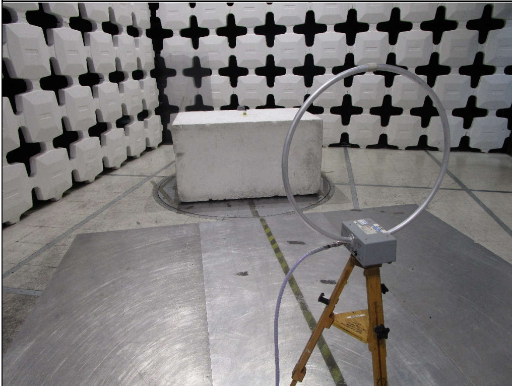
Test Setup for Spurious Radiated Emissions, 150kHz-30MHz – Antenna Polarization Vertical
