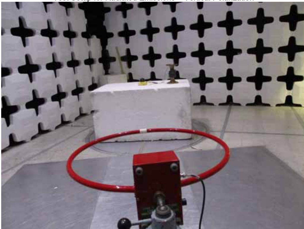
Test Setup for Radiated Emissions – Horizontal Polarization
