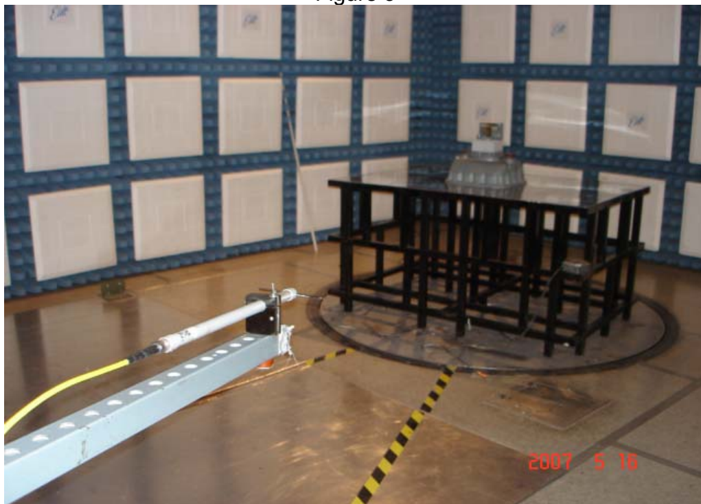
Test Set-up for Radiated Emissions, 911.65MHz to 921.25MHz Horizontal Polarization
