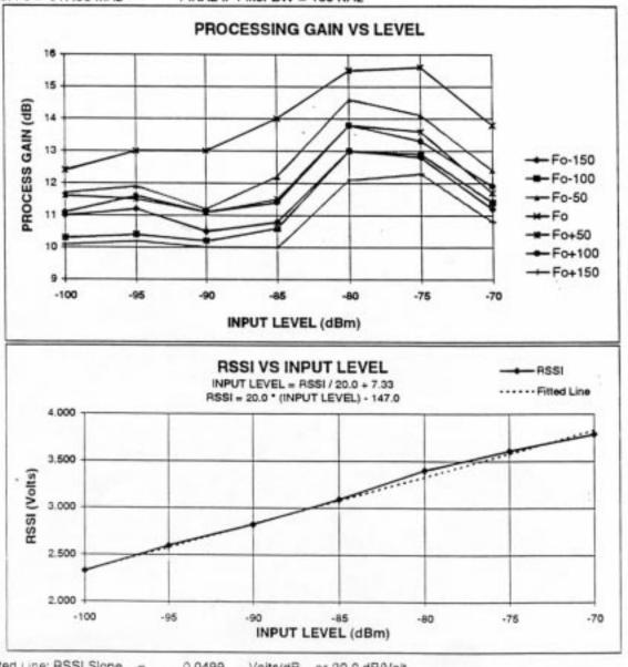
Fitted Line: RSSI Slope = 0.0499 Voits/dB or 20.0 dB/Volt RSSI Intercept Pt. = 7.330 Volts
