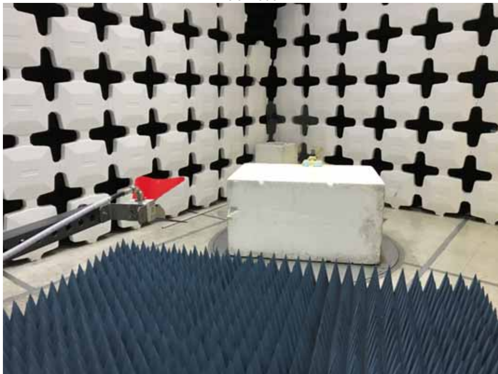
Figure 6 – Receiver Test Setup for Radiated Emissions – 1GHz to 10GHz, Vertical Polarization
