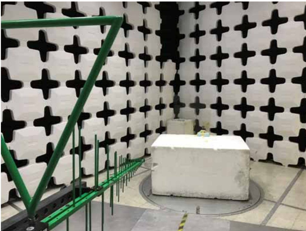
Figure 4 – Receiver Test Setup for Radiated Emissions – 30MHz to 1000MHz, Vertical Polarization
