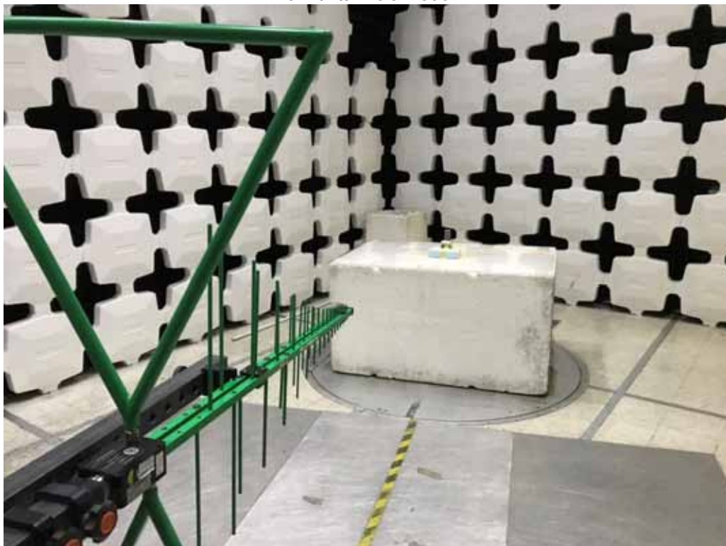
Figure 8 – Transmitter Test Setup for Radiated Emissions – 30MHz to 1000MHz, Vertical Polarization
