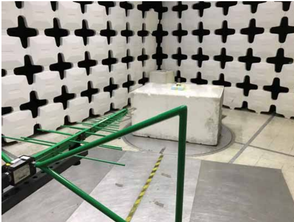
Figure 7 – Transmitter Test Setup for Radiated Emissions – 30MHz to 1000MHz, Horizontal Polarization
