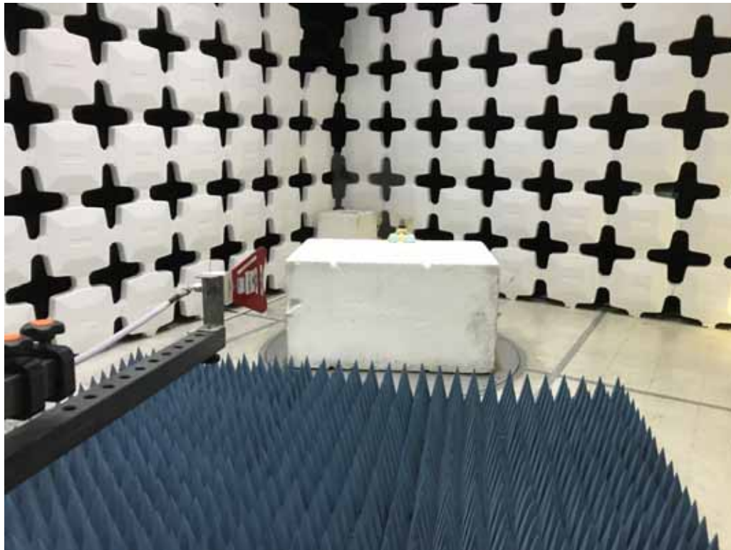
Figure 5 – Receiver Test Setup for Radiated Emissions – 1GHz to 10GHz, Horizontal Polarization
